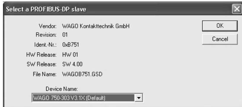
Fig. 6-8: Selecting the PROFIBUS-DP slave
